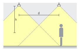
**General lighting**As an approximate luminaire distance (d) between two luminaires, the height (h) of the luminaire above the working plane can be used. The intersecting beams produce excellent uniformity. The recommended offset from the wall is half the luminaire spacing.
