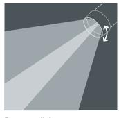
**Zoom spotlights** The light beam diameter can be infinitely adjusted from spot (15°) to wide flood (65°) by simply turning the lens. Zoom spotlights are particularly suitable for illuminating areas with changing exhibits and merchandise.
