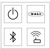
Control types The track can be used for various methods of control: switching, dimming, DALI, Zigbee or Casambi
