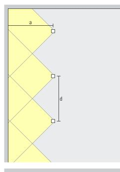
Accentuation Quinta recessed spotlights effectively accentuate works of art, merchandise and architectural details. The ideal angle of tilt ( $\alpha$ ) for this is around 30°. The object is modelled without distorting the effect as a result of excessive shadowing. It also prevents shadows cast by the observer.
