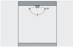
**Display case lighting** Semi-recessed luminaires are particularly discreet and can be installed in the showcase ceiling and floor. Mounting frames for one, two or four light heads are optionally available.
