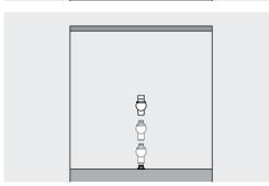
**Display case lighting** Axis stem luminaires and surface-mounted luminaires can be supplemented with additional, magnetically attachable light heads. This creates flexible lighting solutions for a variety of different exhibits. Up to 2 extension light heads can be added when mounting on the floor and one when mounting on the ceiling.
