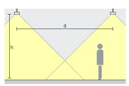
**Linear lighting**Mounted in a row, the oval beams generate linear illumination, for example for circulation areas in the office or for hallways. As an approximate luminaire distance (d) between two luminaires, 1.5 times the height (h) of the luminaire above the working plane can be used.
