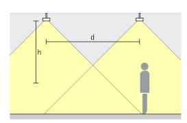
**General lighting**To achieve a high level of uniformity and good facial recognition when illuminating office workstations, up to 1.5 times the height (h) of the luminaire above the working plane can be used for the spacing (d) between two luminaires. The intersecting beams produce excellent uniformity. The recommended offset from the wall is half the luminaire spacing.
