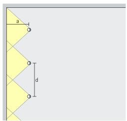
For good longitudinal uniformity, the luminaire spacing (d) of Optec wallwashers may be up to 1.2 times the distance to the wall (a).
