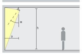
Wallwashing For uniform vertical illuminance, the distance (a) of Opton lens wallwashers from the wall should be around one third of the room height (h). This results in an angle of tilt ( $\alpha$ ) of approx. 35°.
