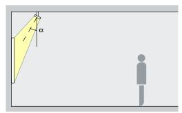
**Accentuation** Opton spotlights accentuate artwork, products and architectural details effectively. The ideal angle of tilt ( $\alpha$ ) for this is around 30°. The object is modelled without distorting the effect as a result of excessive shadowing. It also prevents shadows cast by the observer.
