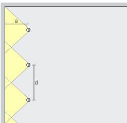
For good longitudinal uniformity, the spacing (d) of Quintessence lens wallwashers may be up to 1.3 times the offset from the wall
