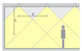
**General lighting**For uniform ambient lighting with high visual comfort, the spacing (d) between two Quintessence downlights may be up to approximately 1.5 times the height (h) of the luminaire above the working plane.
